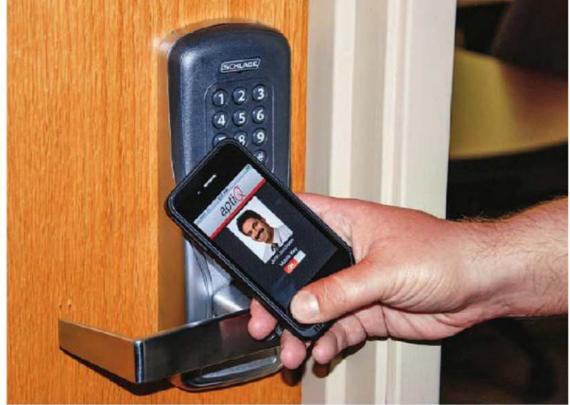
Cell phone is used as a personal security key with Schlage AD-Series Lock. Photo courtesy Ingersoll Rand Security Technologies.
